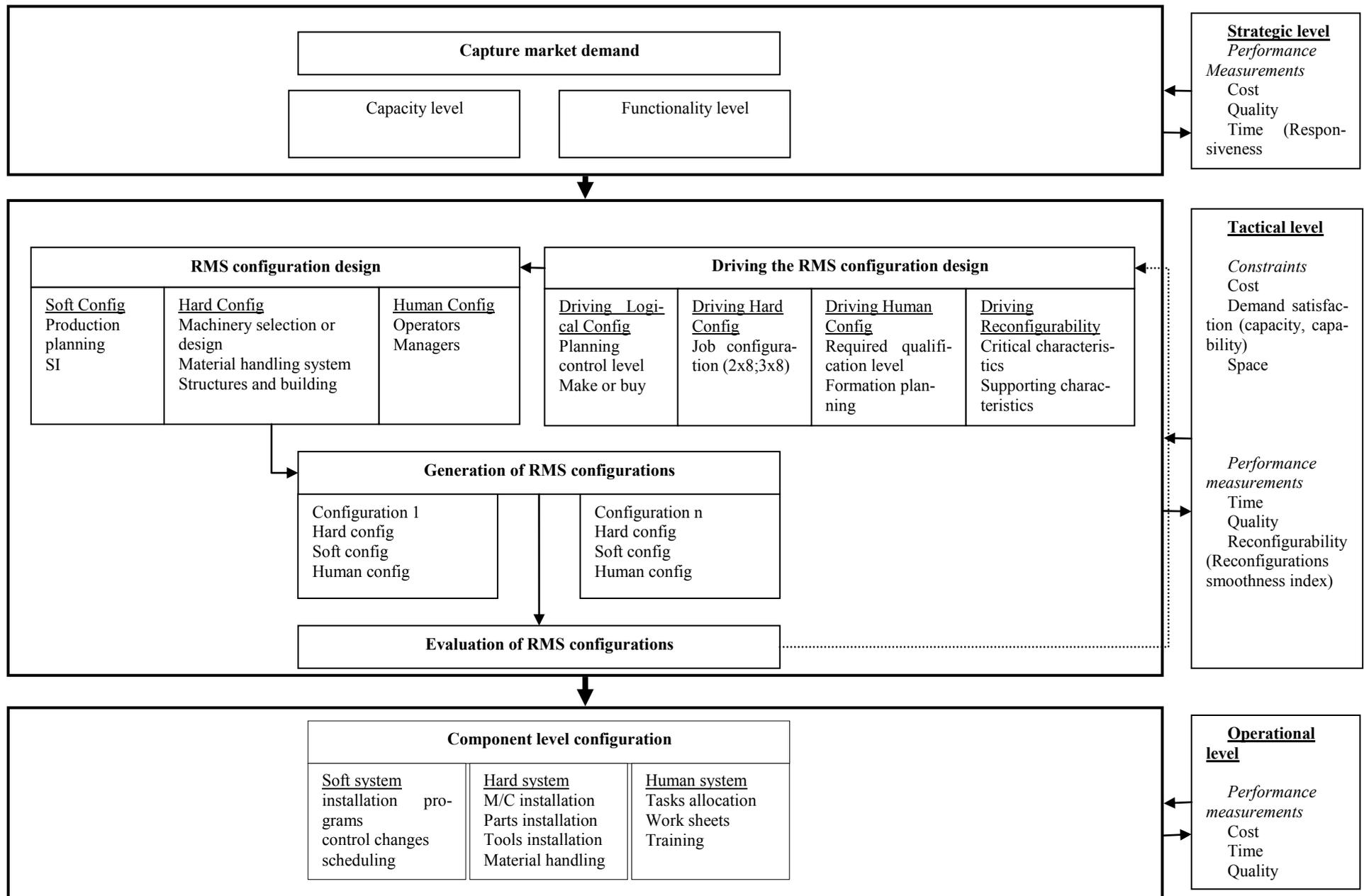
Fig. 2. : Reconfigurable manufacturing system design framework
