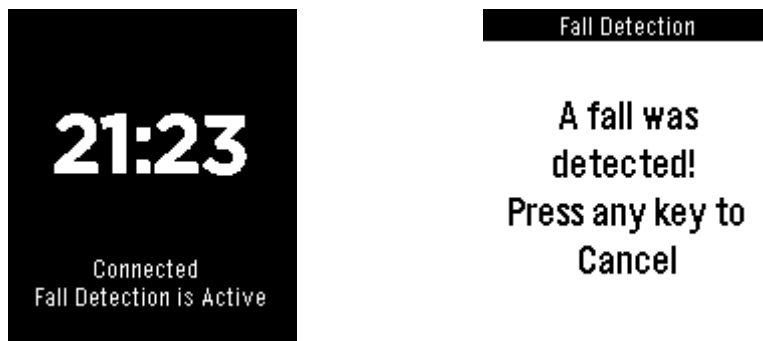
Figure 3. Screenshots of the Pebble Smart watch Application in case of an idle active connection and in case of a detected fall
