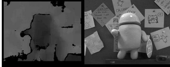
Fig.5. Depth map from stereoscopic camera device
