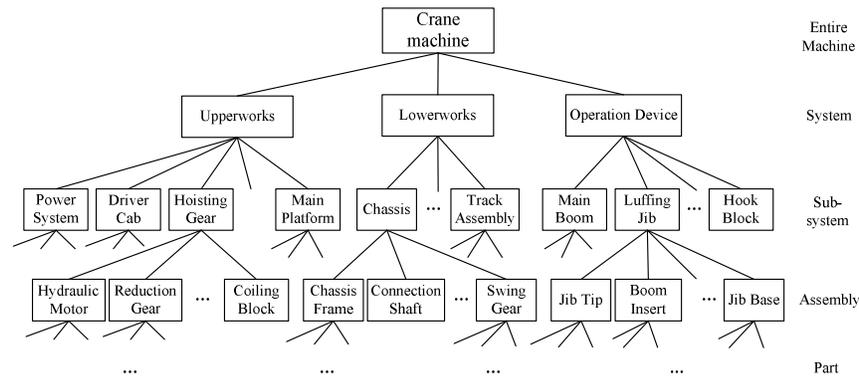
Fig. 3. The hierarchical structure of a crane machine.
