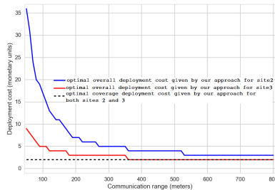
Fig. 3: Optimal deployment cost given by our approach depending on the communication range of nodes.
