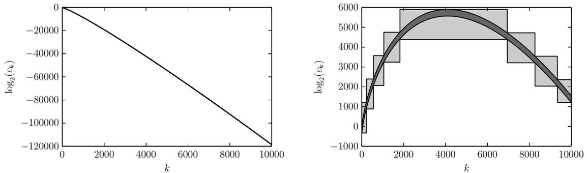
Fig. 1. Transformation used to square  $\exp(x) = \sum_k x^k/k! \in \mathbb{R}[x]/\langle x^n \rangle$  with  $n = 10^4$  at  $p = 333$  bits of precision. The original polynomial, shown on the left, has an effective height of  $\log_2(n!) + p \approx 119\,000$  bits. Scaling  $x \rightarrow 2^{12}x$  gives the polynomial on the right which is split into 8 blocks of height at most 1511 bits, where the largest block has a width of 5122 coefficients.
