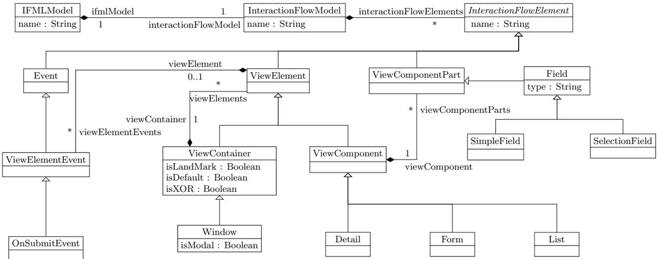
Figure 1: Simple Ecore model of an IFML subset.
