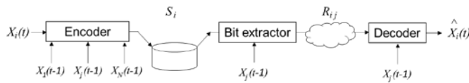
Fig. 7. Mixed: partial (perfect) knowledge of the previous request at the encoder (sender, respectively).
