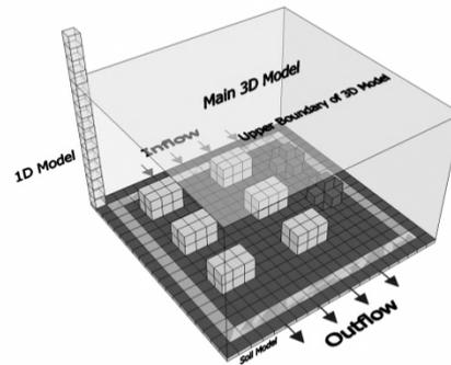
**Fig. 2.** The schematic overview of the model layout
