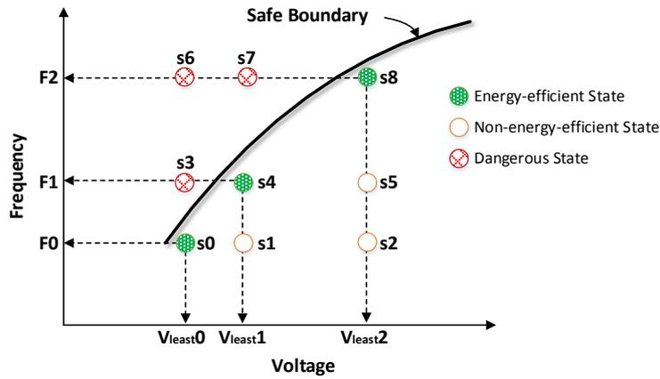
**Fig. 1.** Dangerous states causing hard faults during DVFS
