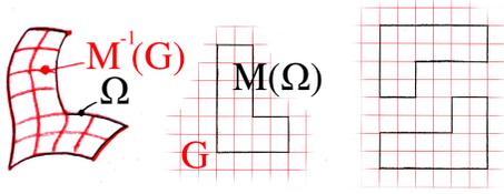
Fig. 3: Considering a bijective continuous map  $M$  from an object  $\Omega$  (left) to  $\mathbb{R}^3$  (center), it is possible to generate a hexahedral mesh of  $\Omega$  by tracing the preimage of the regular grid from  $\mathbb{R}^3$  (center) to the object. Note that a whole family of maps – that we call “grid-equivalent” – produces exactly the same hexahedral mesh (right).
