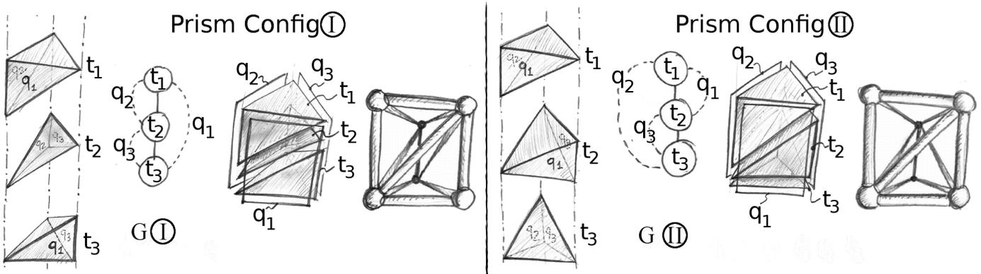
Fig. 25: For a fixed front quadrilateral face ( $q_1$ ), there are two decompositions of a prism into three tetrahedra, from left to right, in exploded view, graph representation, compact view and shaded wireframe.
