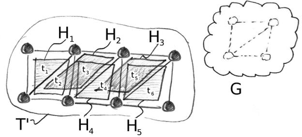
Fig. 10: Recombination (in 2D): the template  $G$  describes the recombination of two triangles into a quad. Five instances  $\mathbf{H}^* = \{H_1, H_2, H_3, H_4, H_5\}$  can be found in the intermediate mesh  $T'$ . Clearly,  $H_2$  and  $H_3$  are of lower quality (lower value of function  $Q$ ).  $H_1$  and  $H_2$  are mutually incompatible ( $C(H_1, H_2) = 1$ ) because they have  $t_2$  in common. The other mutually incompatible pairs are  $(H_2, H_4)$ ,  $(H_4, H_3)$  and  $(H_3, H_5)$ .
