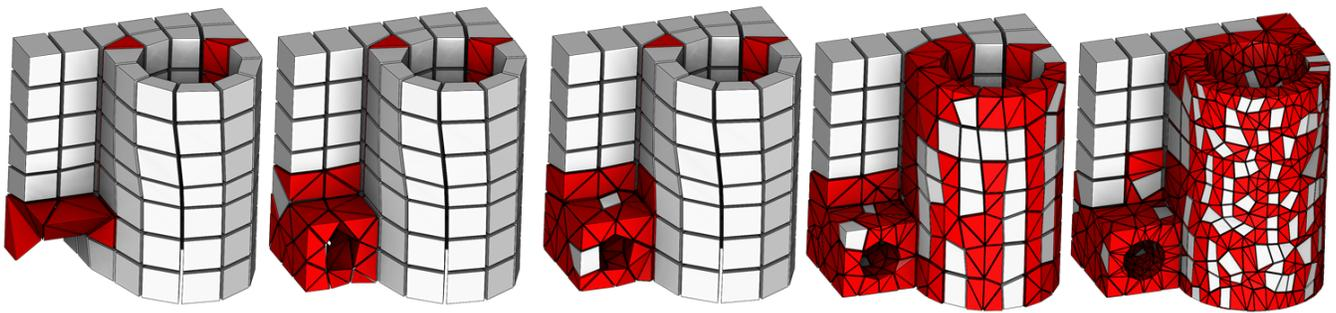
Fig. 15: Influence of the maximal deviation parameter  $\epsilon \in \{100\%, 2\%, 1\%, 0.5\%, 0.25\%\}$  of the average edge length of the input mesh. A high tolerance misses some features (left), whereas a too strict tolerance inserts too many points (right).
