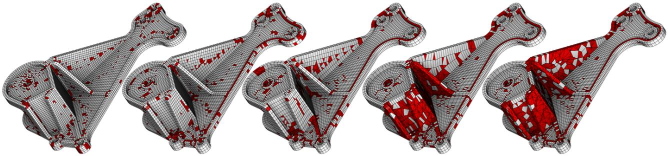
Fig. 14: Influence of the maximum curl-correction parameter  $\gamma \in \{1, 0.8, 0.6, 0.4, 0.2, 0\}$ . A value of  $\gamma$  that is too low results in the same over-constrained problem as in CubeCover (right images).
