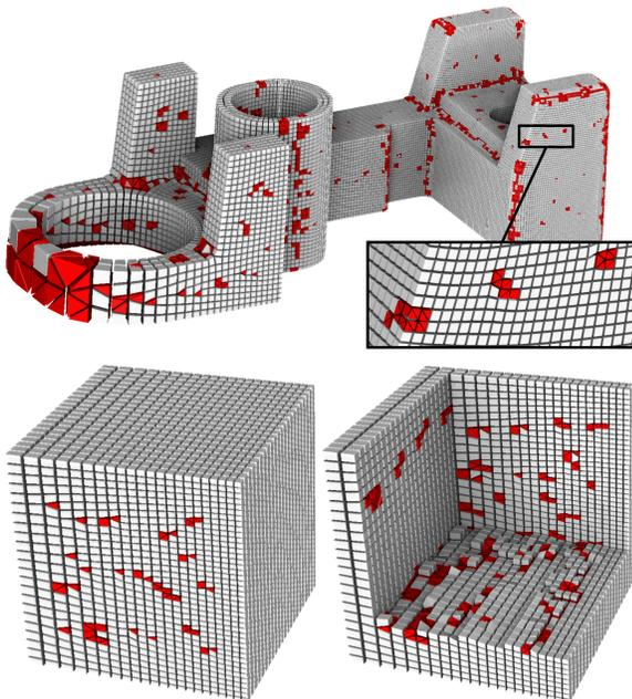
Fig. 16: Varying scale: In the upper image, the desired hexahedra size varies linearly with the  $x$  coordinate. The bottom row shows a cube (clipped on the right image) with a varying anisotropic scale. Singularities are evenly distributed to absorb the variation of resolution.
