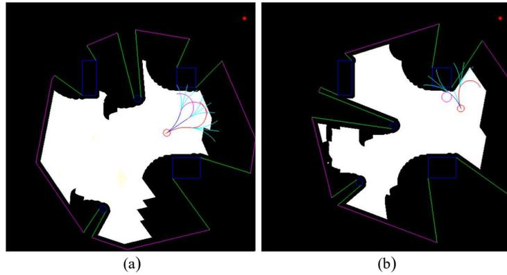
**Fig. 5.** P-safe RRT trees corresponding to the second (a) and third snapshot (b) of figure 4. Tree's primitives represented in blue are p-safe, those in cyan are  $ICS^b$  (not p-safe) and those in magenta characterize collision-free braking trajectories (for each  $ICS^b$  node, a braking trajectory is generated). The selected trajectory (to be executed) is represented in red.
