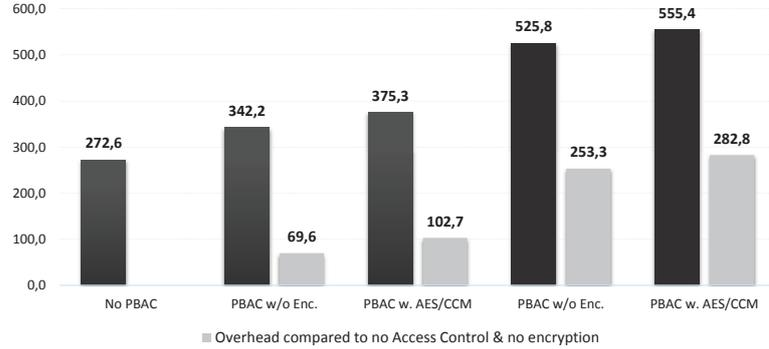
**Fig. 3.** Response time (in ms) for a single request, averaged over 50 data points. Columns in dark gray depict the scenario where there is no security between the sensor and the Provider, while black columns correspond to the scenarios where AES-CBC encryption was used to protect said link.
