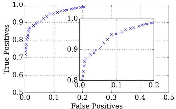
**Figure 3:** Receiver operating characteristic for wireless bottleneck detection.
