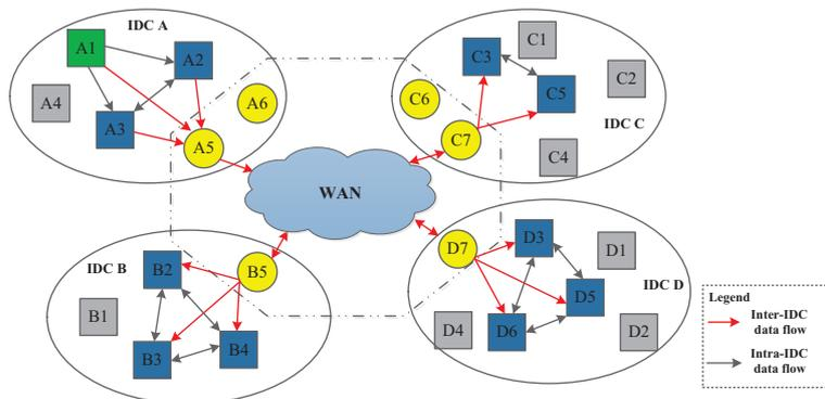
**Fig. 1.** The brief diagram of bridgehead-employed distribution mode
