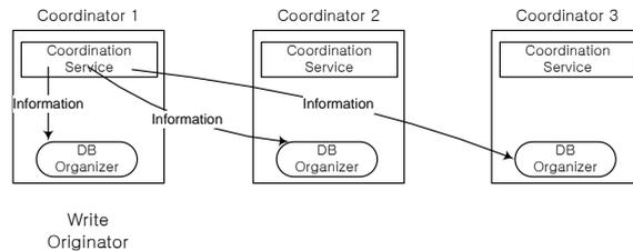
**Fig. 3.** Information writing to the management DB of the other coordinators are acknowledged later and the coordination service continues without these acknowledgements.
