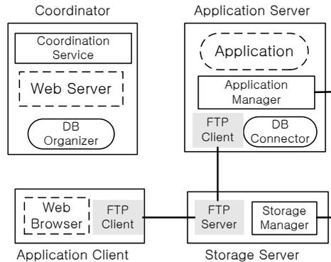
**Fig. 1.** System architecture of the computing Grid
