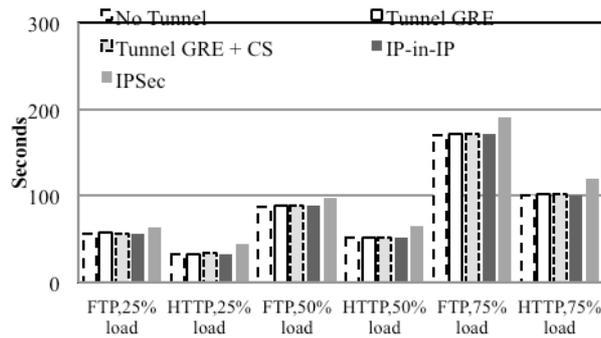
**Fig. 2.** Shows the end-to-end delay of the examined tunnelling techniques (CS=Checksum)
