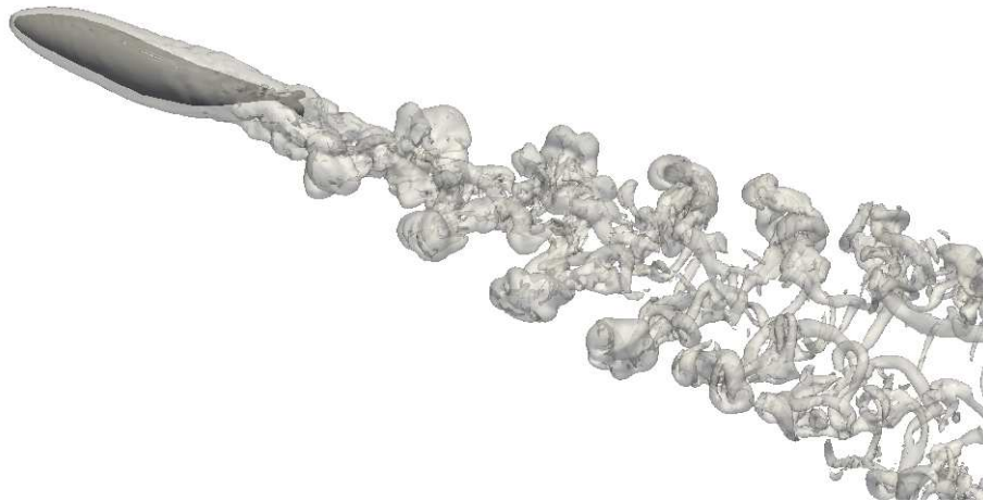
Figure 12: Isovorticity representation of the wake generated by the mackerel fish starting from actual pictures.
