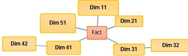
**Fig. 1.** Snowflake schema in multidimensional data model
