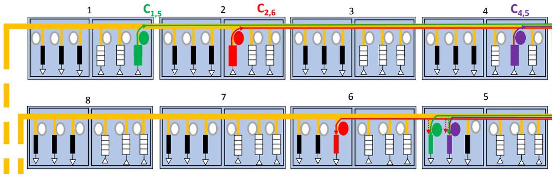
FIGURE 4 – Optical elements state in ONoC for MWD at the 65th second
