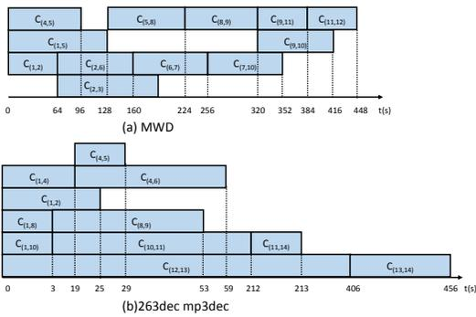
FIGURE 2 – Communication details for MWD and 263dec mp3dec
