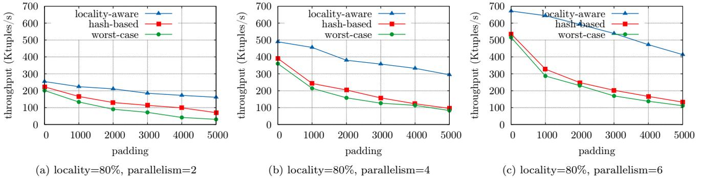
Figure 9: Throughput when varying tuple sizes, with a locality of 80% and different parallelisms
