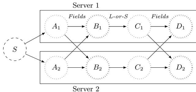
Figure 3: Deployment of a stateful streaming application, with fields grouping linking POs  $A$  and  $B$ , local-or-shuffle grouping linking POs  $B$  and  $C$ , and fields grouping linking POs  $C$  and  $D$ .
