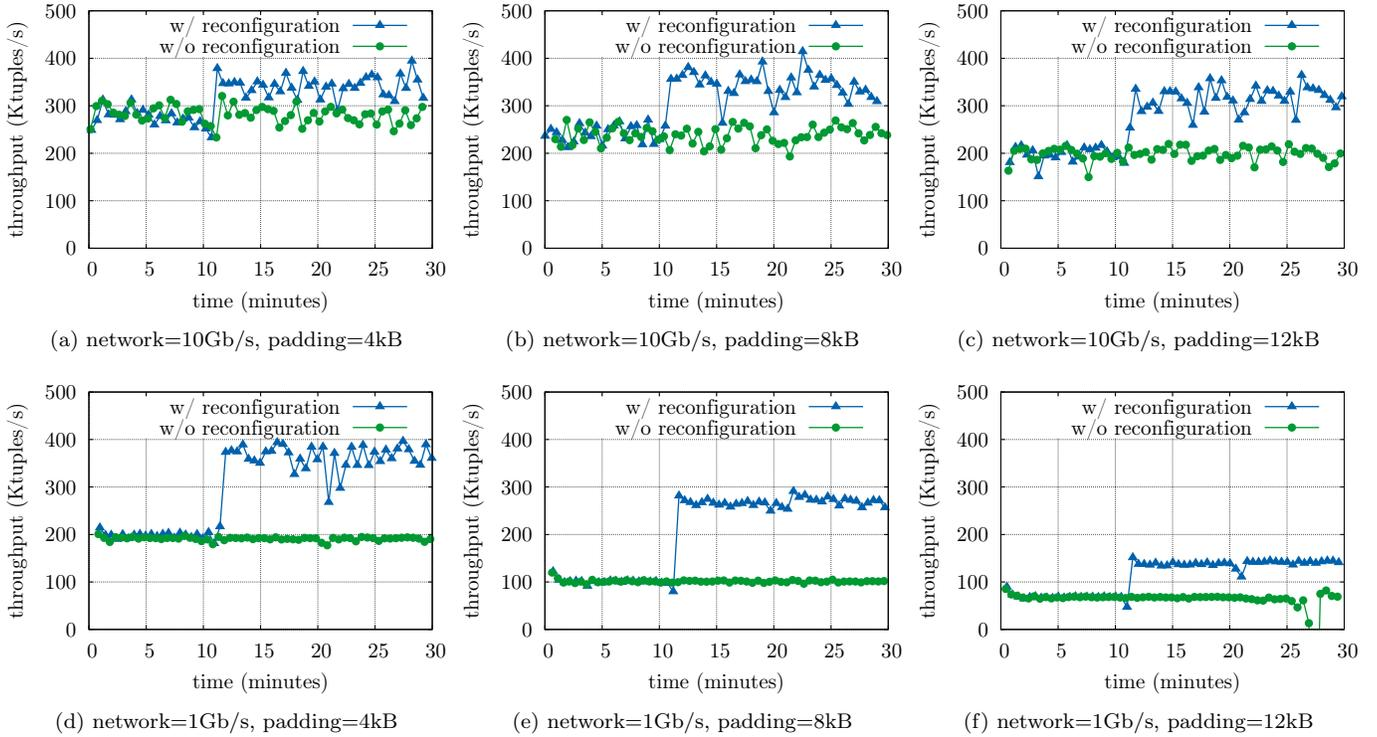
Figure 13: Evolution of the throughput with or without reconfiguration, for a parallelism of 6, different padding sizes and two types of network bandwidth.
