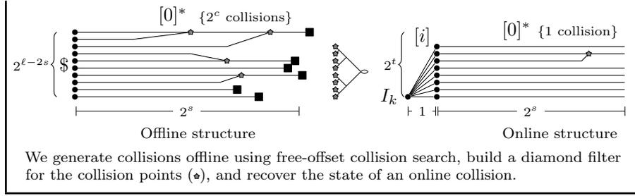
*Complexity analysis.* In Step 1, we use free-offset collision search with  $2^{\ell-2s}$  starting points and chains of length  $2^s$ , and thus according to Section 3.1, we find  $2^{\ell-2s}$  collisions (*i.e.*  $c = \ell - 2s$ ). Furthermore, according to Lemma 3,  $\hat{y} \in \hat{X}$  with high probability, in which case the attack succeeds.
