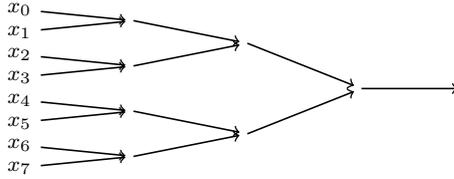
Once we finish building the diamond structure, we construct a standard collision filter for the final node  $y$ , using message blocks  $([b], [b'])$ . Thus, building a diamond filter offline for  $2^t$  states requires  $O(2^{(\ell+t)/2})$  time, which is faster than the  $O(2^{t+\ell/2})$  time required to build a collision filter for each node separately.
