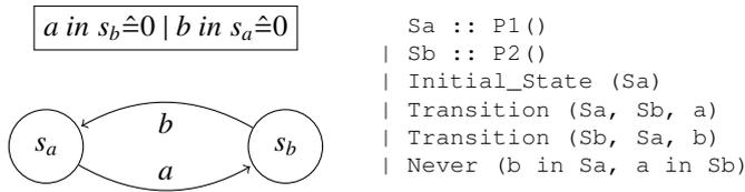
Figure 7 “alternate” automaton
