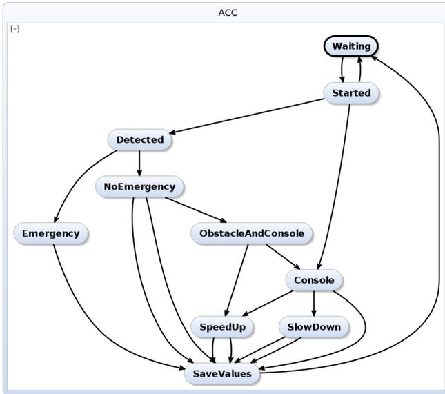
**Figure 14** State transition system for the *ComputeActionThread* thread.
