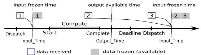
Figure 8 Execution time model for an AADL thread
