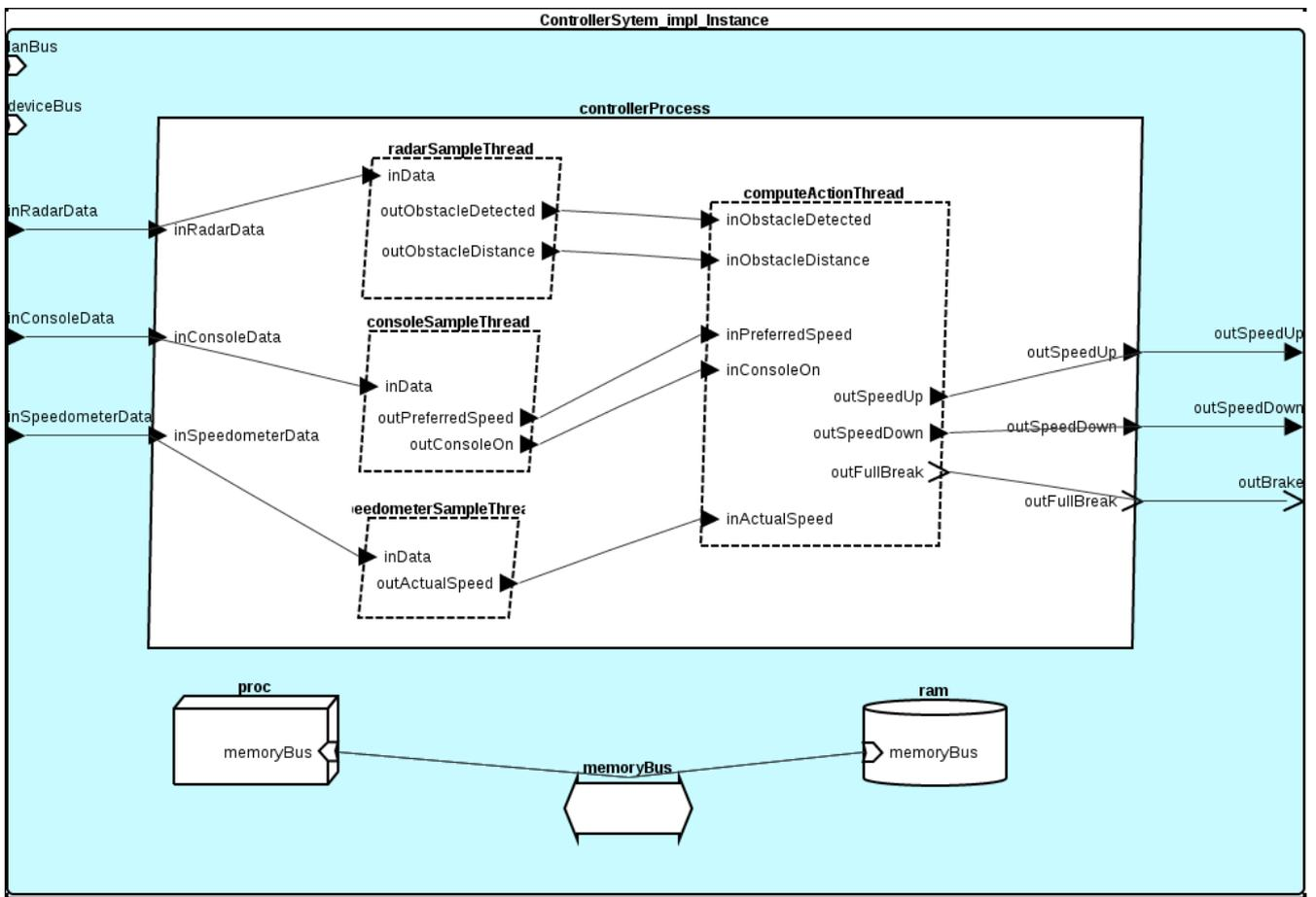
**Figure 13** Controller subsystem of the Adaptive Cruise Control system modeled with AADL. Rectangles represent processors, double-arrows buses, cylinders memories and rhombuses processes and threads.
