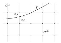
Fig. 9: Complete stencil for the discretization of the Neumann boundary condition.
