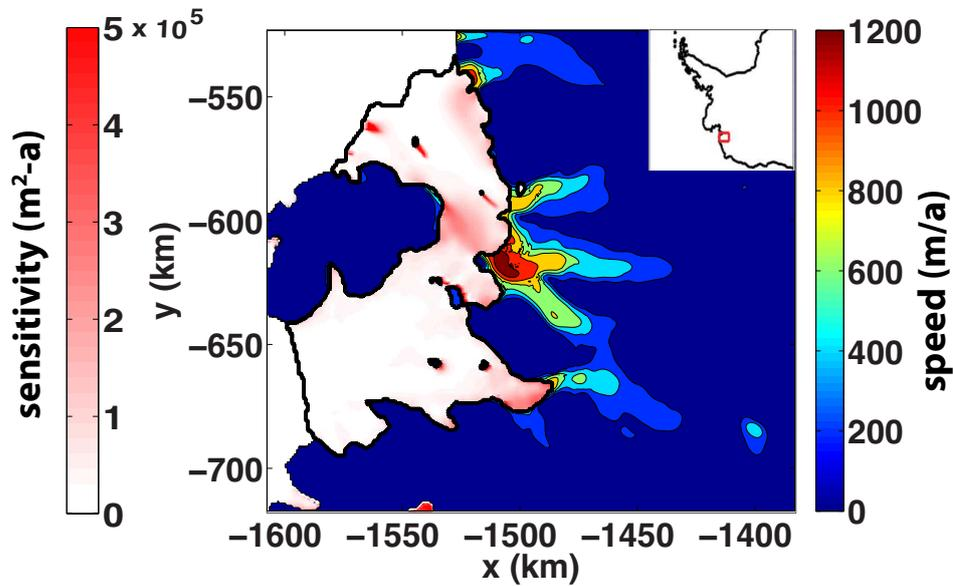
**Figure 3.** Adjoint sensitivity of loss of Volume above Floatation (VAF) to basal melting under the ice shelves adjacent to Smith Glacier (location shown in inset). Filled contours give modeled ice velocity where ice is grounded; red-white shading gives adjoint melt rate sensitivity under ice shelves. The thick black contour denotes the boundary of the ice shelves.
