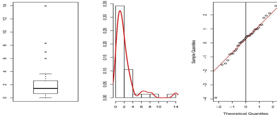
Figure 7: Case 2 (38 hydrogen flow rates): Boxplot (left), histogram with a smoothed-kernel density function (middle) and quantile-quantile plot with respect to a log-normal distribution.
