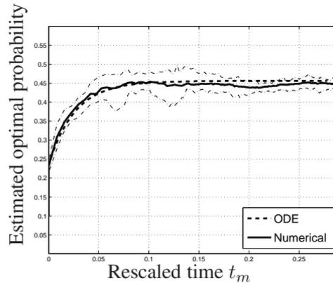
Figure 3: The convergence of the dynamics of the control variable against the reference ODE; at the time scale  $t_n$  and averaged over 10 sample trajectories in the case of static control. Thin dash-dotted lines delimit the maximum and minimum values attained by the estimate trajectories.
