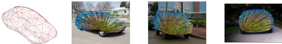
Fig. 1. Our approach models a three-dimensional object in terms of a graphical model, where the nodes correspond to 3D part positions and the edges encode geometric constraints between part positions. Given an input image and a viewpoint estimate the cost function of our energy model dictates the optimal placement of the parts in three dimensional space , obtaining a reconstruction of the object’s surface from a monocular image.
