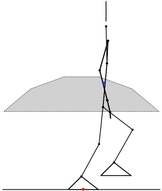
Fig. 2. The maximal reachable region of the CoM of the robot  $c$  (blue dot) with respect to the center of the support foot  $p$  (red dot) usually has a nonlinear shape, but this shape can be very well approximated by a convex polyhedron, here in gray.
