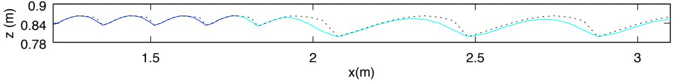
Fig. 3. Trajectory of the CoM of the robot in the sagittal plane when walking on a flat, even ground, transitioning from a speed of  $0.2 \text{ m.s}^{-1}$  (dark blue) to a speed of  $0.6 \text{ m.s}^{-1}$  (light blue). The dotted curve is the kinematic limit due to maximal leg length. When the step length increases with speed, the maximal CoM height during the double support phase lowers significantly, resulting in a more pronounced vertical motion of the CoM.
