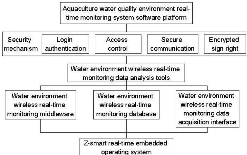
Fig. 1. Structure Design of System Software Platform
