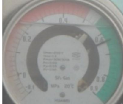
Fig.2 . Color image of SF6 pressure gauge
