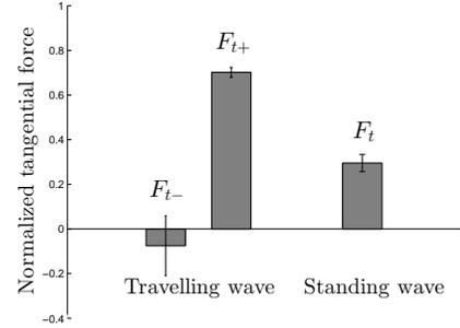
Fig. 9. Low friction level with a travelling wave and with a standing wave at  $1.6 \mu\text{m}$
