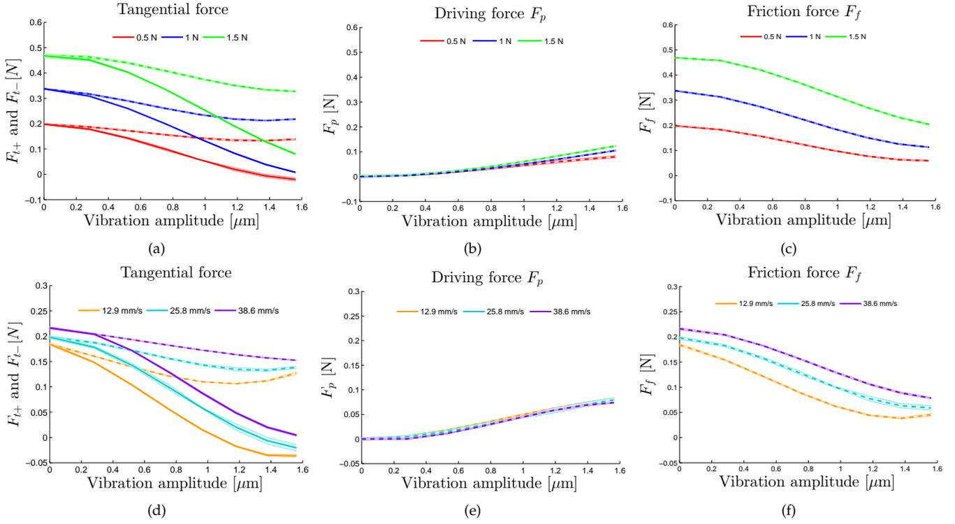
Fig. 6. Tangential forces (first column,  $f_{t+}$  dashed line, and  $f_{t-}$  plain line), driving forces (center column), friction forces (last column), for various normal force  $F_N$  (top) and various velocities  $v$  (bottom). The shadowed area near the measures represents the standard deviation for each measures.
