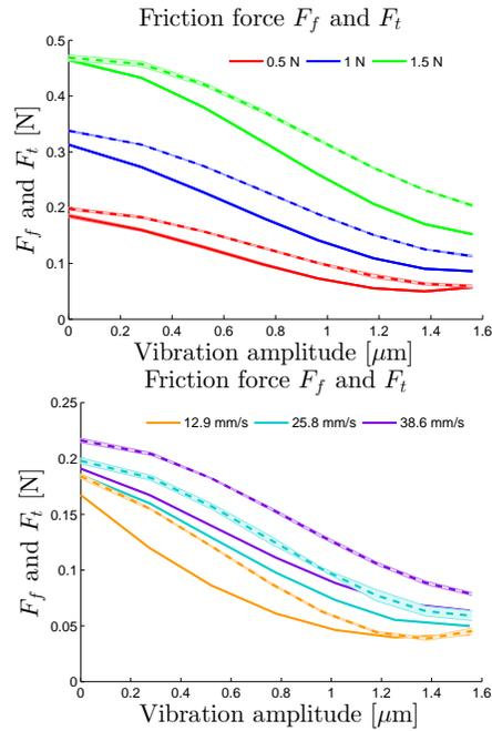
Fig. 10. Tangential forces for a standing wave (plain line) compared to the friction force  $F_f$  of the travelling wave (dashed line) for several normal force (top) and velocities (bottom) conditions.
