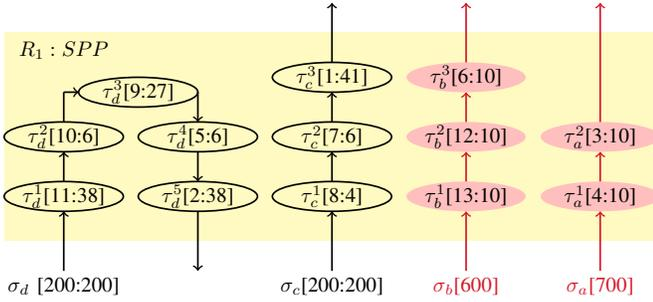
Figure 4. Model of our case study. We use the following notations: task chains are specified as  $\sigma[\delta^-(2) : D]$  and tasks with  $\tau[\pi : C]$ . Chains  $\sigma_c$  and  $\sigma_d$  are periodically activated while  $\sigma_a$  and  $\sigma_b$  are sporadic, overload chains.
