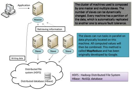
Figure 1: Set up of the Cloud architecture.
