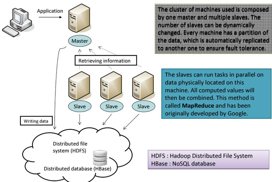
Figure 1: Set up of the Cloud architecture.
