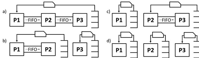
Fig. 2. Four options for a three-process system with FIFO lanes and supermarkets
