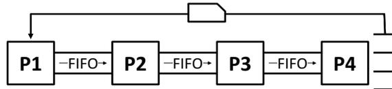
**Fig. 1.** Example of a four process kanban system with FIFO lanes and supermarkets using standard value stream mapping nomenclature
