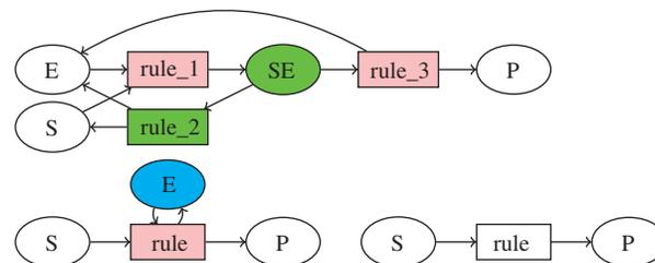
**Fig. 1.** Reaction graphs of the Michaelis–Menten enzymatic reaction, either complete with intermediary complex  $SE$ , or reduced with or without enzyme  $E$ . The first reduction can be achieved with the graphical operations explained in Section 2.2, for example by merging the reaction nodes  $rule\_1$  and  $rule\_3$  in pink into a reaction node  $rule$  and by deleting the green nodes  $SE$  and  $rule\_2$ . The second reduction simply deletes the blue node  $E$ .
