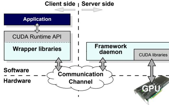
**Fig. 1.** Architecture usually deployed by GPU virtualization frameworks.
