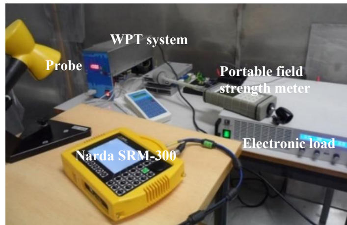
Fig. 3. WPT system - Experimental setup.
