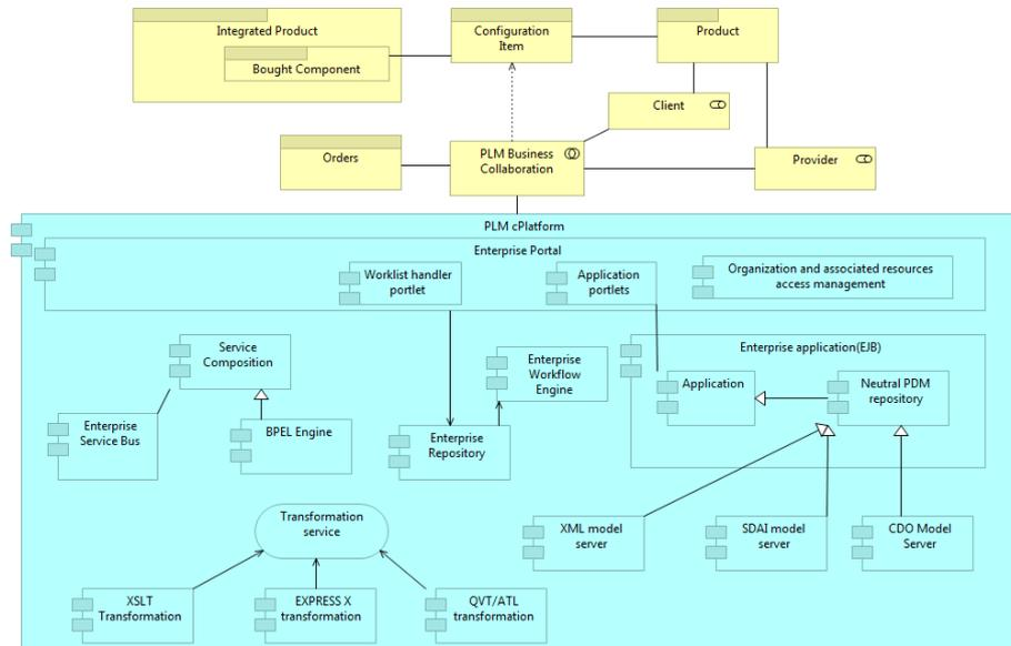
**Figure 2: ArchiMate model for cPlatform and supported collaboration**
