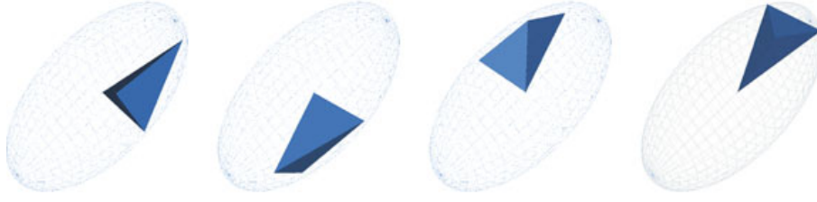
Fig. 2 Some unit-elements with respect to a 3D metric represented by its unit-ball
