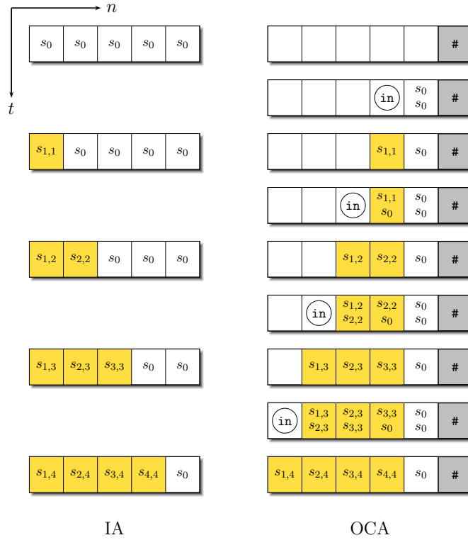
Fig. 4. Simulation of two-way information flow by one-way information flow. The input to the OCA is provided at the cells marked by the circled in.
