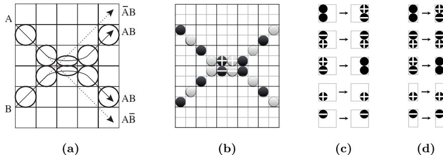
**Fig. 1.** Scalable Soft Sphere dynamics. (a) Stroboscopic view of continuous classical collision, one time step per column. (b) Finite state collision, with particles drawn lighter at odd time-steps. (c) 2D partitioning rule. Only these cases (and their rotations) interact. Otherwise, all particles move diagonally, unchanged. (d) 1D version of the rule.
