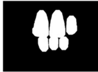
Fig 6.b. After applying Opening on Fig 5
