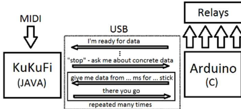
Fig. 4 Data flow diagram
