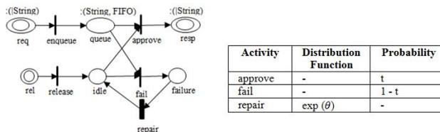
**Fig. 5.** HCSAN model of the hardware resources
