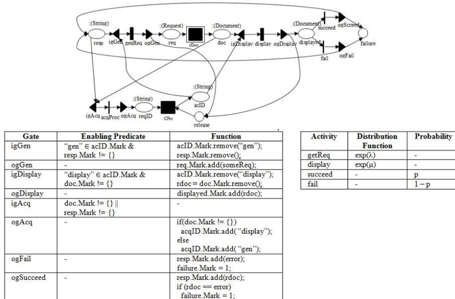
Fig. 2. HCSAN model of *CApp*
