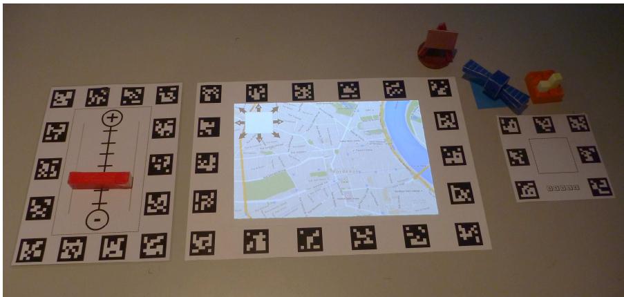
Figure 2. Photograph of an interactive geographic map for sighted people implemented using the PapArt OpenSource framework and hardware. The prototype projects a map on a paper sheet, and provides tangible, touch-based and spatial interaction techniques (Chatain et al., 2015). In the VISTE project we aim at extending this prototype with supplementary non-visual cues (e.g., audio output).
