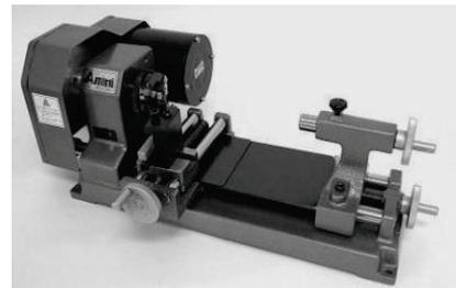
Figure 2. Tabletop lathe
