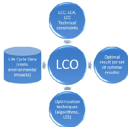
This framework considers three main elements for making a successful LCO: life cycle data, life cycle methodologies and optimization techniques. The presented tool will have the task of converting life cycle data related to environment (like used material, energy consumptions, etc.) in environmental impact. Future development will be the substitution of Eco-Indicator with something of more understandable like the Carbon Footprint.
