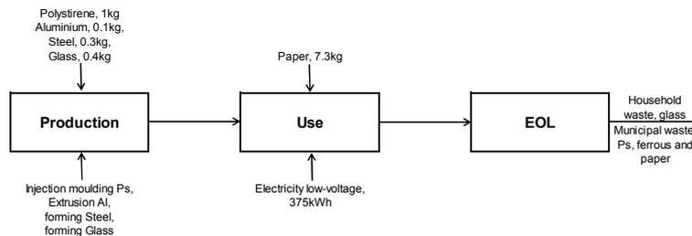
Materials and processes used to realize the coffee machine are considered, while in the Use phase filter papers and electricity to work the coffee machine are evaluated. Finally in EOL disposal of materials is taken into account.
