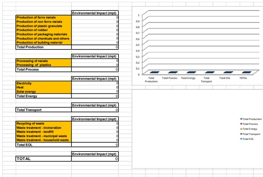
Material, Process, Energy, Transport, EOL and Total environmental impacts are reported. Also a bar and a pie chart are realized to simplify the reading of the results.
