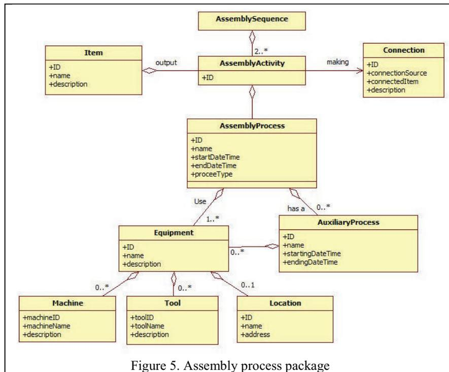
Figure 5. Assembly process package
